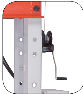
Winch provides easy positioning of press bed
