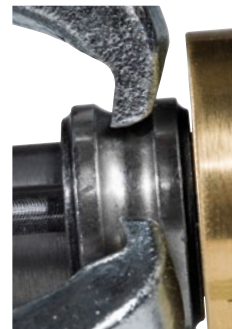
Lock on ball grooves and bearing races.
