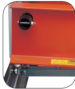
Bearings make bed positioning smooth and easy.
